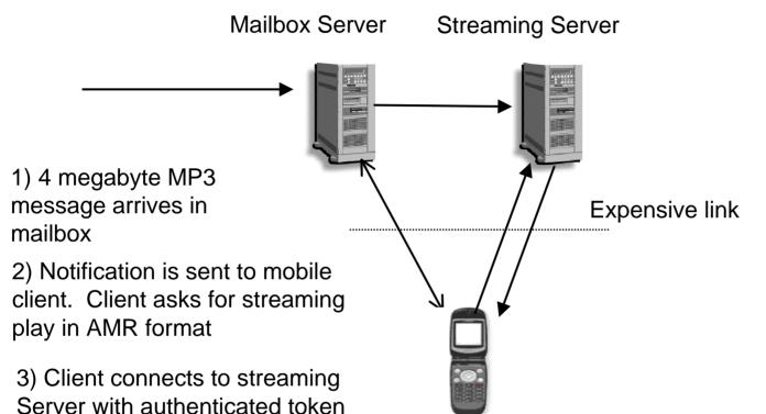
4) Streaming server grabs MP3, Transcodes it, and streams to client
